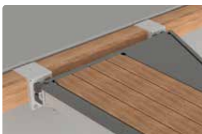
Connection to concrete pontoon.
