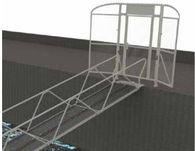
Gate for mounting on the shore abutment.
