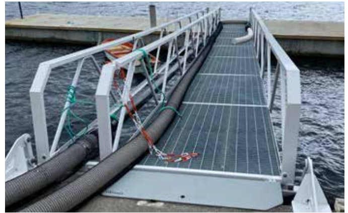
Mowi, Rovde in Vanylven: Gangway, 16 x 2,2 m, with grating deck and an additional side section for easy transport of fish to the boat.
