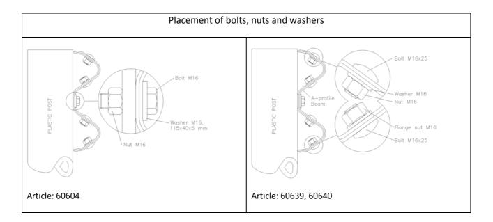
**Note:** Please check that all bolts/fasteners are placed correct and all bolts-washer-nuts-connections are normally/proper fastened/tighten.
