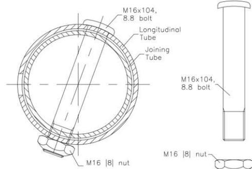
*Exploded view over attachment of longitudinal element to post and section view of joint.*
